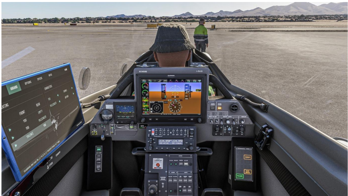
Notice the green “Trainer” indicator on the annunciator panel.
